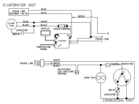
Fig. 2.4 VINO6500SSR Electrical Wiring Diagram (VTSTAT)
